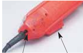
Variable Heat Control Off/On Trigger
