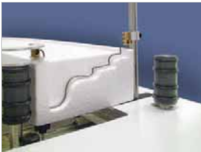
Cut Compound Curves and Negatives for Precast Concrete
