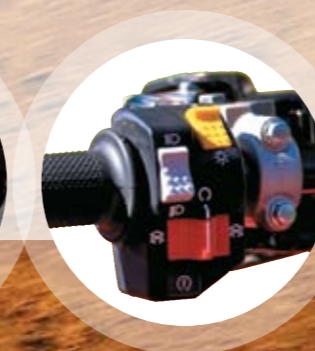
Electric starter for easy starting in all conditions.
