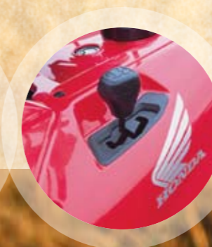
A shift selector gives the choice of standard output ratios (Drive) and reverse.
