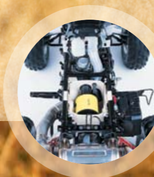
Standard TRX air-intake filtration system picks up fresh air from the highest point on the ATV.
