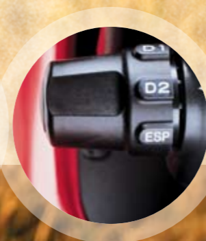
Dash-mounted switches allow you to shift quickly between six different Hondamatic™ transmission variables.
