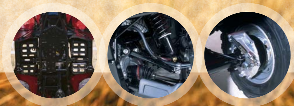
Front and rear premium shock absorbers provide 150mm of travel for ultra-comfortable all day riding.
