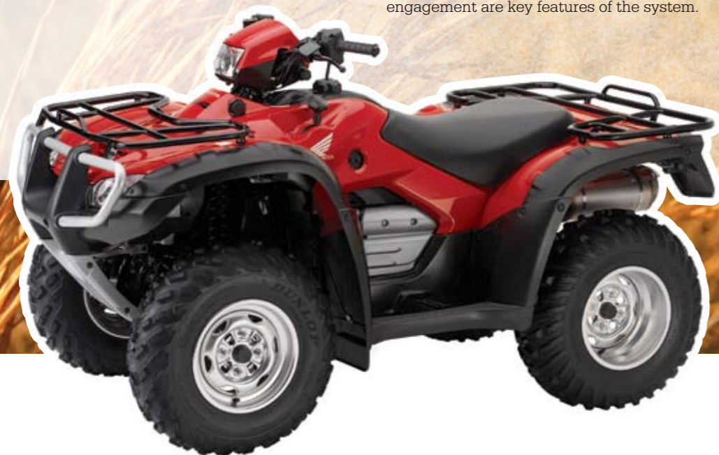
Independent double-wishbone front suspension and swingarm.
