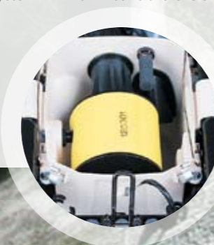
TRX air-intake filtration system picks up fresh air from the highest point on the ATV.
