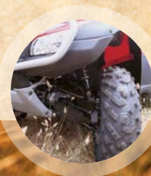
Independent double-wishbone front suspension and swingarm.
