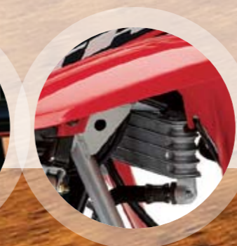
High-efficiency oil cooler supplements the large-capacity oil tank for maximum engine cooling.
