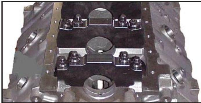
Beefy bottom end has solid rails, choice of nodular iron or splayed main caps.
