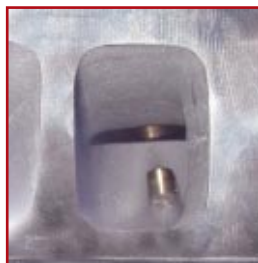
The 80cc Combustion Chamber Is Unique To The Merlin-X Head Highly Effective 350cc intake Ports
