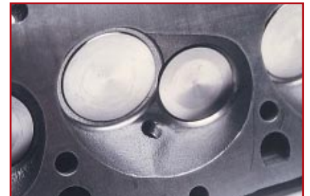
119cc "Open" Chamber Design Is Far Superior To OEM "Closed" Chambers
