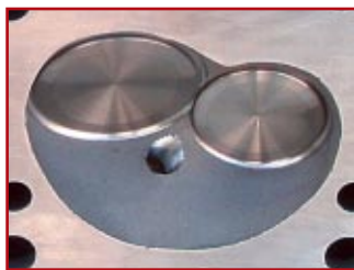
Highly Efficient 119cc Combustion Chambers
