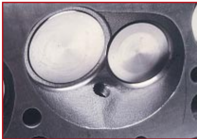
119cc "Open" Chamber Design Is Far Superior To OEM "Closed" Chambers
