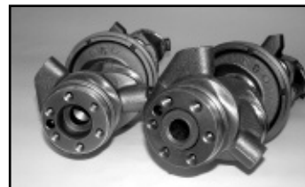
The crankshaft on the right shows the bushing that Hi-Tech includes
