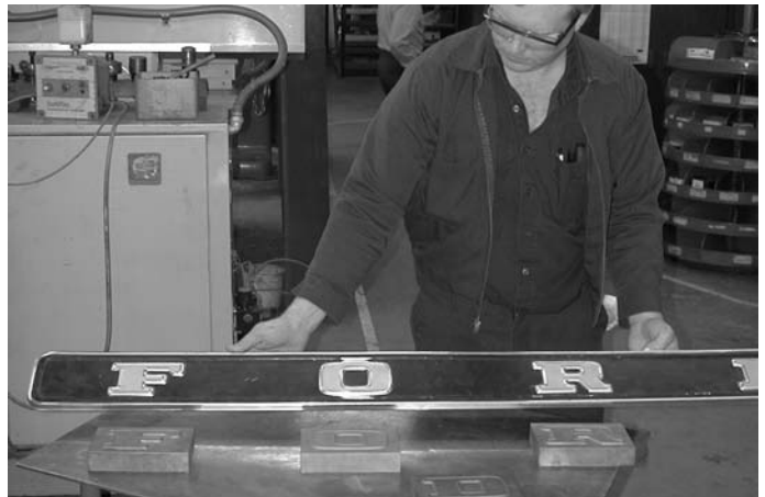
Reid Coggins shows a finished tailgate finish panel. In the foreground are the A-2 tool steel male form blocks which are used to stamp the Ford letters into the aluminum panel.
