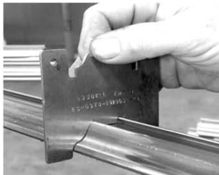
The molding contour is regularly checked for accuracy
