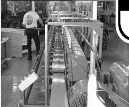
Aluminum stock is drawn through a series of roll forming dies
