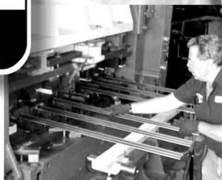
Some stamping tools will do several operations simultaneously like this 7 stage arrangement.
