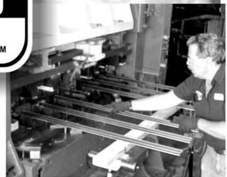
Some stamping tools will do several operations simultaneously like this 7 stage arrangement.
