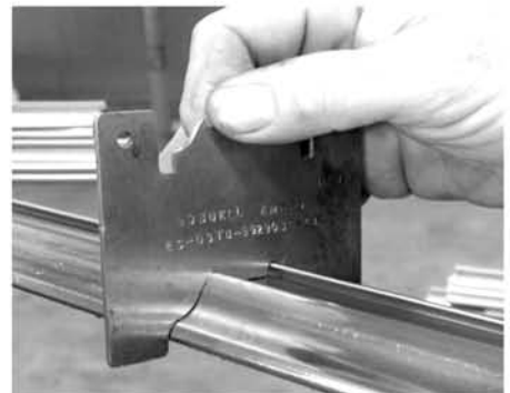
The molding contour is regularly checked for accuracy
