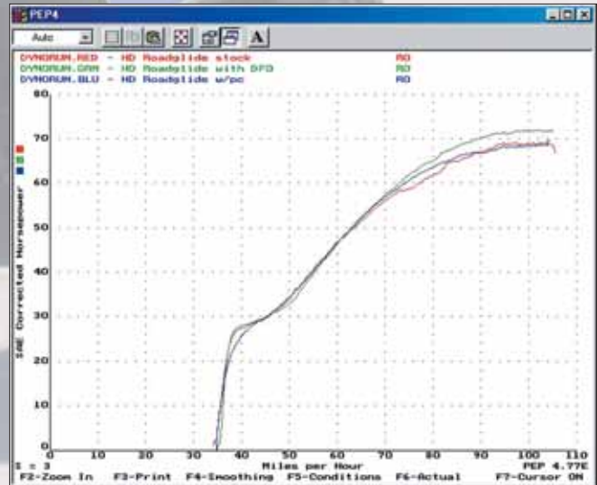
The Red run is a stock EFI Road Glide. The Blue run is with a Power Commander installed. The Green run is with the DFO added.
