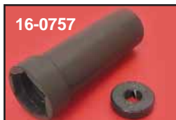
Countershaft Sprocket Lock Nut Wrench features an extra long two piece design inner collar which will retain wrench to nut. Fits 1936-up Big Twins, 1 7/8" hex, 4 and 5 speed models.
