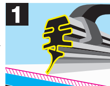
Wiping action makes windshield water repellent
