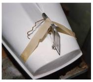
Applying grease into the propshaft tube or "stuffing box" is not always the best idea. A tube packed with grease can create a lot of drag on the rotating shaft, which can slow the motor and cause poor performance and overheating. It is recommended to apply light machine oil to the bearing ends.
