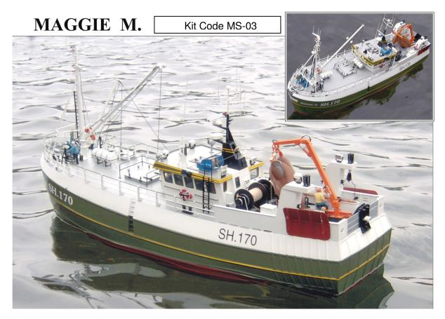
Built in 1990 by Campbeltown Shipbuilders Ltd (Scotland) MAGGIE M operates out of Scarborough harbour in Yorkshire, United Kingdom. The vessel is designed for twin-rig trawling and the aluminium shelter deck is a cover over the fish processing room. The shelter deck allows the trawling to be undertaken in virtually all seas, the winch being controlled from the back interior of the wheelhouse thus minimizing the exposure by the crew to the weather elements.
