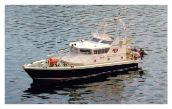
The kit is designed as an introduction to the skills and techniques of constructing a model boat from a glassfibre hull and styrene parts for the cabin, with major fittings either vacuum-formed from styrene or cast in alloy.
