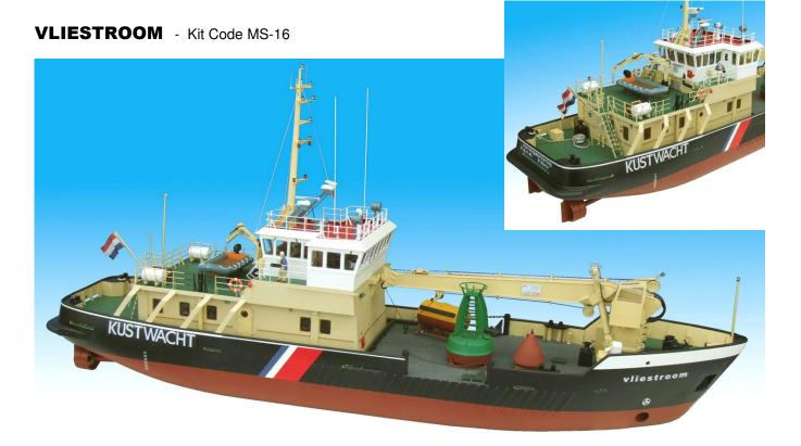
*Vliestroom* and her sister ships *MV Nieuwe Diep* and *Schuitengat* were built by Damen Shipyards in 1987-90 for the Dutch Ministry of Transport and Waterways. The folding main mast and cantilevering radar masts together with the low draught flat-bottomed hull allow for a very versatile craft, which can encounter low bridges and shallow waters in and around Holland. This unusual and distinctive model is based on *Vliestroom*, built in 1987, operating out of Hellevoetsluis.
