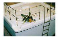
Always place a clip lower down near the plastic deck to dissipate the heat away from it, as you do not want it melting and making the hole in the deck bigger.
