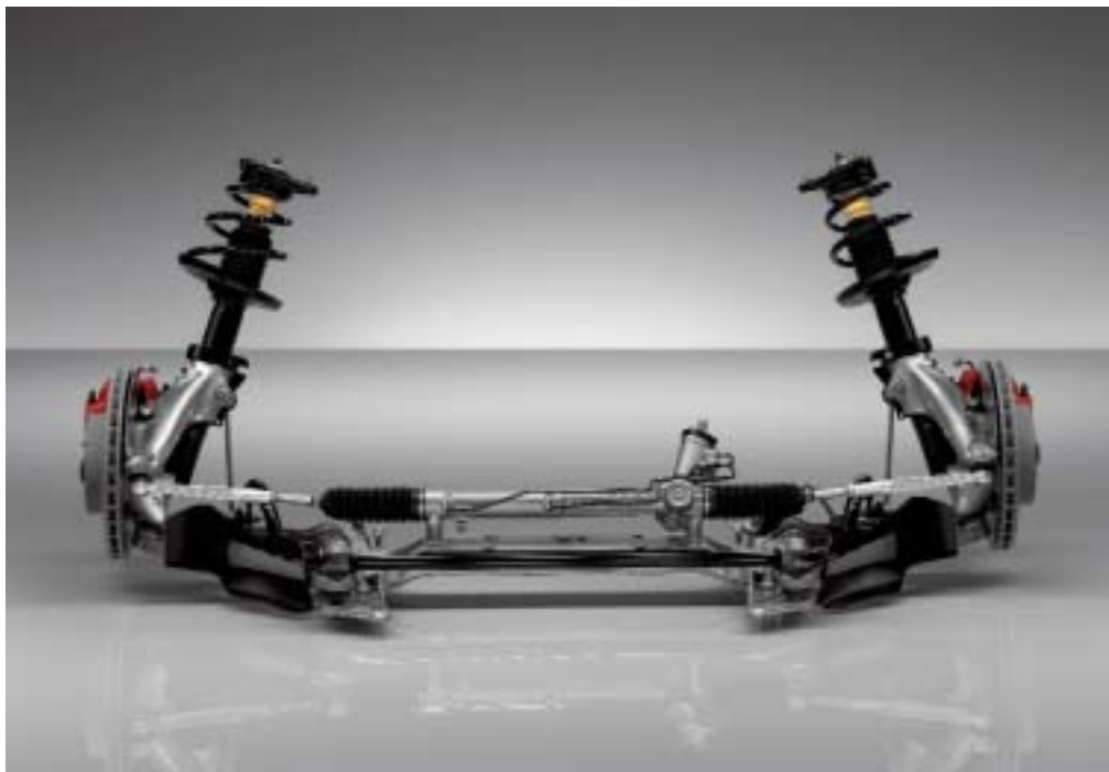
Front axle with McPherson struts and lateral control arms
