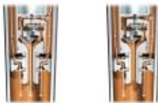
Left: Rebound in 'Normal' mode – bypass valve open Right: Rebound in 'Sport' mode – bypass valve closed
