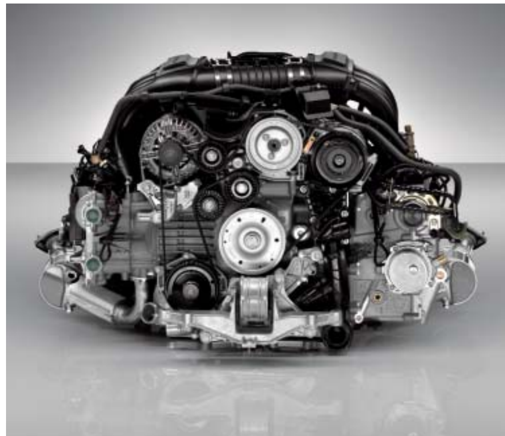
3.4-litre six-cylinder boxer engine
