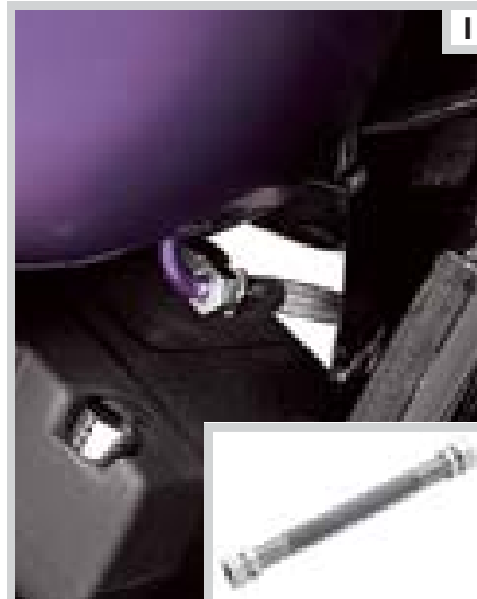
I. BRAIDED STAINLESS STEEL FUEL CROSSOVER LINE
