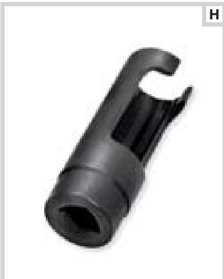
H. SCREAMIN' EAGLE AUTOMATIC COMPRESSION RELEASE REMOVAL TOOL
