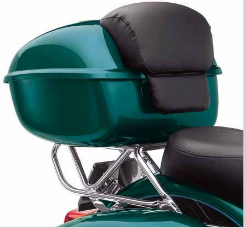
A. COLOR-MATCHED SPORT TOUR-PAK LUGGAGE (SHOWN WITH DETACHABLE TOUR-PAK RACK AND PASSENGER BACKREST PAD)
