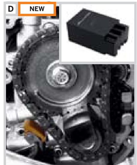
D. SCREAMIN' EAGLE CAM LOCKING TOOL – SILENT CHAIN
