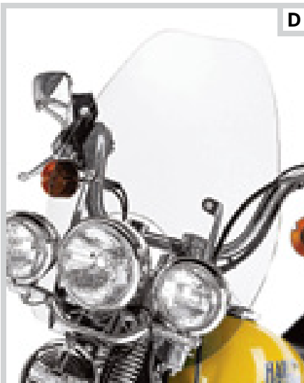
D. DETACHABLE SUPER SPORT WINDSHIELD FOR FX SPRINGER SOFTAIL MODELS – 13" LIGHTLY SMOKED
