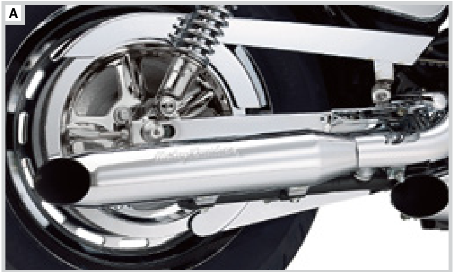
A. CHROME SWINGARM (SHOWN WITH CHROME UPPER AND LOWER BELT GUARDS AND CHROME SPROCKET COVER)
