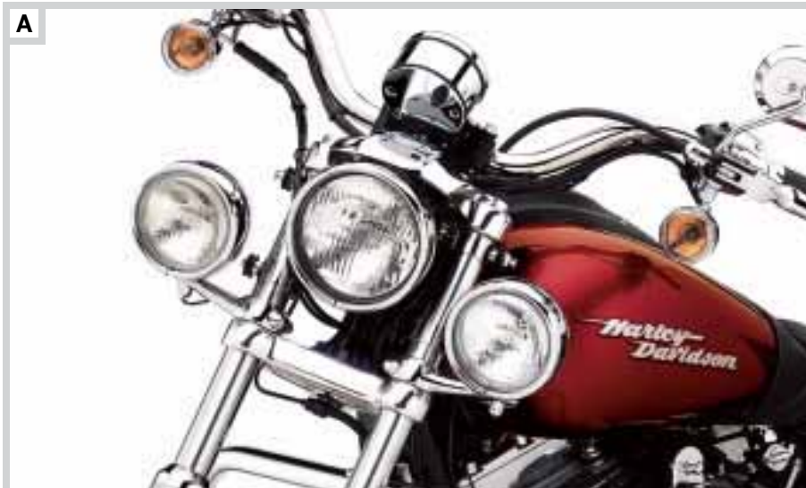
A. AUXILIARY LIGHTING KIT – SPORTSTER/DYNA (SHOWN WITH AUXILIARY LAMP BULB KIT – CLEAR WITH LENS OPTICS)
