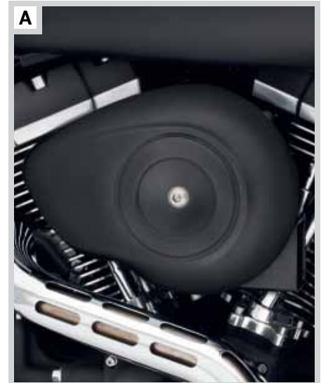
A. AIR CLEANER COVER FOR TWIN CAM MODELS ('08-LATER DYNA SHOWN) – PRIMED (CUSTOM PAINTED)
