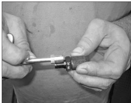
Male & female threads can be checked using the BrakeQuip Thread Gauge #BQ2100
