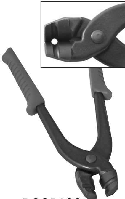
1 Brake Tube Pliers allows a tight 90° bend on the brake tube, right at the tube nut.
