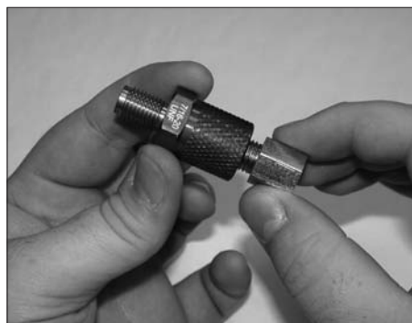
Male & female threads can be checked using the BrakeQuip Thread Gauge #BQ2100
