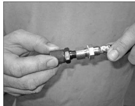
Male & female threads can be checked using the BrakeQuip Thread Gauge #BQ2100
