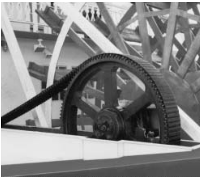
Paddle wheel drive on a large riverboat
