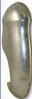
1947-48 RH Front is same as LH rear and LH front is same RH rear.
