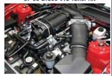
The VTS 3300 twin screw compressor is capable of supporting 900+ horsepower & over 22 psi of boost. Kit Includes: 4.0" 10-rib compressor pulley, billet adapter plate, integrated bypass valve assembly, custom PCV adapter & Maxflow cast aluminum supercharger air inlet.
