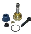
Steeda's X5 ball joints improve suspension geometry on lowered Mustangs by raising the spindle relative to the ball joint pivotpoint. This raises the rollcenter back into the correct range for optimum handling.
