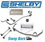
Sway bars are post-assembly heat treated chromoly steel & include polyurethane bushings. Front bar is 35mm with 3 endlink mounting points for a wide range of tuning possibilities. Rear sway bar is 22mm thick with gold anodized 7075-T6 billet aluminum endlinks with 12.9 grade hardware & nylocks. '05-11
