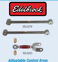
Features a urethane bushings on one end, and a spherical ball joint on the other end to eliminate bushing bind. Can be adjusted to fine tune pinion angle.
