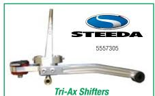
CNC-machined from 6061 aluminum, stop bolts prevent over travel, potentially saving your transmission's life. Factory steel mounting rail is replaced with a billet beam for more positive location. Retains factory shift boot and shift knob. Lifetime warranty.
