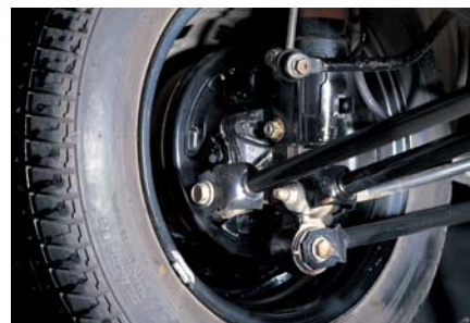
Lubricating the rubber cups of auto brakes
