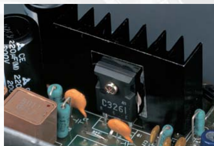
Heat dissipation for power transistors
