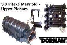
This Improved Intake Manifold has reinforced wall material in failure-prone areas for excellent durability. This greatly resists cracking where the O-E does not, especially at the throttle body coolant passage where the EGR gases corrode the walls of the coolant passage.
