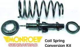
These kits replaces all four air struts. This kit is fully engineered to be a complete and thourough conversion of the suspensin structure. It has been engineered to not interfere with the vehicles other ECU's and not drain the elecronics. It is necessary that instructions be followed to insure that no electronic warning signals result.
