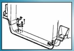
15.5" core supports (or sometimes referred to as non-AC-style) have a bottom cross-rail shaped like an up-side-down "U".
