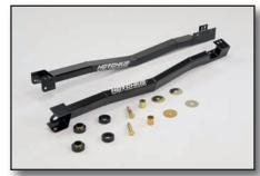
Made from 1.5" x 2.5" x .120" wall steel tubing. These come black powder coated. Includes urethane front mounts. Rear mount needs to be welded in and front can be either bolted or welded. Floor pan mods are not required.
