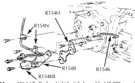
R154A 1964-67 Backup Light Switch Assembly, MT (RP)..... 29.00/ea. This universal switch assembly bolts on the shifter and is activated by the reverse arm. Although not of original design, it is an inexpensive alternative to R154B and R154D.
