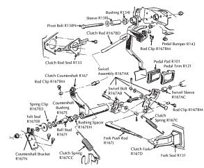
Typical 1968-72 A-Body Clutch Linkage
