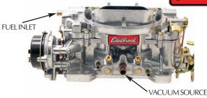
The Performer Series carburetors from Edelbrock feature two-piece all-aluminum construction for cooler fuel and less warpage. There are no gaskets below the fuel bowl level to leak and no plastic parts or power valves to blow out. The primary venturi feature is a bottom-feed design for improved drivability and smooth acceleration. These carbs use easily changeable metering rods for precision-tuning.
