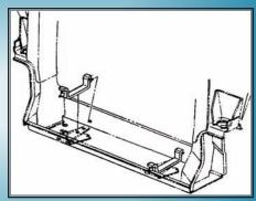
17.5" core supports (or sometimes referred to as AC-style) have a bottom cross-rail shaped like an right-side-up "U".
