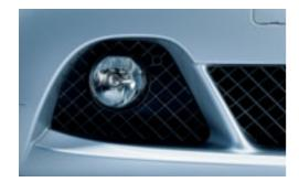
■ Halogen free-form foglights are cleanly integrated into the front bumper, illuminating the road ahead in bad weather.
