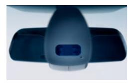
■ Rain sensor uses infrared light to measure the amount of rain. When the wipers are in the "intermittent" mode, the rain sensor automatically adjusts the windshield wiping interval as needed. Automatic headlight control (included with rain sensor but not shown), activates the headlights by means of a sensor that responds to darkness.
