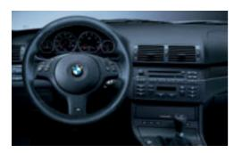
M three-spoke leather-wrapped multi-function sport steering wheel has fingertip cruise, audio and accessory phone<sup>1</sup> controls.
