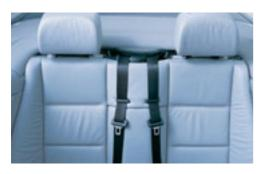
■ Three-point safety belts at both rear seating positions hold occupants comfortably and safely in place.
