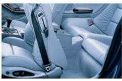
■ Ingenious seatback easy-entry feature offers power fore/aft controls that may be used to move the seat forward all the way for easy access, then back again to the seat's original position. Each front seat has two sets of fore/aft controls – the controls on top move the seat double-speed, for quickest access.
