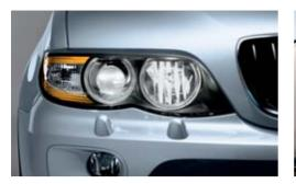
**Xenon Adaptive Headlights** optimize road illumination when entering a curve or bend, helping to enhance safety when driving at night. Sensors continuously monitor the vehicle's driving data to determine the direction and how much to swivel the headlights – up to 15 degrees to the left or right. (std. in X5 4.8is and X5 4.4i; opt. in X5 3.0i)
