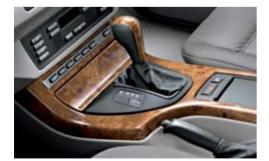
**STEPTRONIC automatic transmission** provides a choice of three modes: "Drive," which incorporates BMW's Adaptive Transmission Control; "Sport" automatic, for a more dynamic shift pattern; and STEPTRONIC automatic, for the hands-on control of a manual without using a clutch. (5-speed STEPTRONIC automatic transmission opt. in X5 3.0i; six-speed STEPTRONIC automatic transmission std. in X5 4.8is and X5 4.4i)
