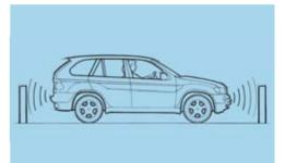
**Park Distance Control** uses eight sensors – four in front, four in the rear – to help you judge how close you are to other cars and unseen objects when parking. The warning beeps become faster as the bumper approaches the object, turning into a constant tone when the distance is less than 12 inches. (std. in X5 4.8is and X5 4.4i; opt. in X5 3.0i)
