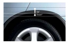
**Adjustable Ride Height** raises the vehicle 1.5"<sup>1</sup> to help protect the undercarriage of the X5 when driving over rough roads, and lowers the vehicle 0.8"<sup>2</sup> when stopped to ease entry and exit. (std. in X5 4.8is; opt. in X5 4.4i and X5 3.0i, and requires Sport Package)
